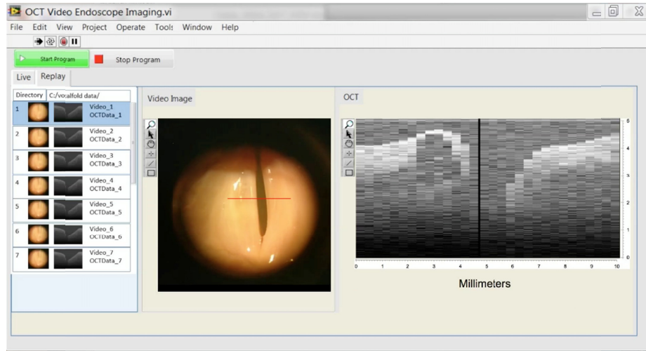
Fig. 8. Mock-up of graphical user interface in stroboscopic OCT-VS mode. The video and OCT data were collected from a phonating human ex-vivo larynx and were combined using post-processing to simulate the display interface [Visualization 1]
