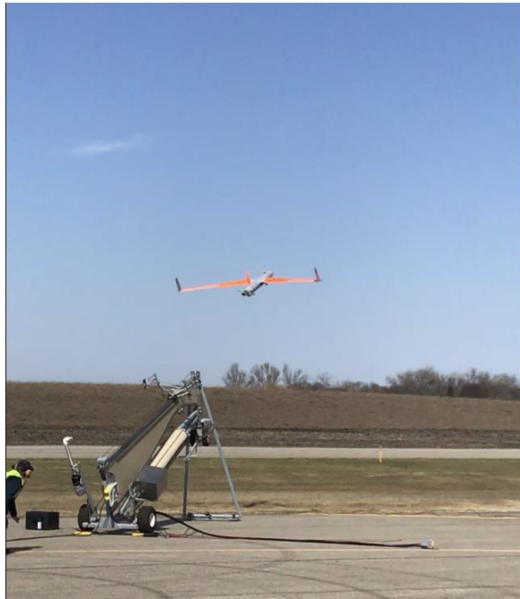
(left) ScanEagle launched (below) ScanEagle recovered with Skyhook
