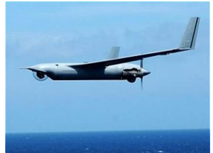
(left) ArcticShark - multipayload capable UAS (right) ScanEagle UAS - used on North Slope - Good endurance 1.2M flight hours
