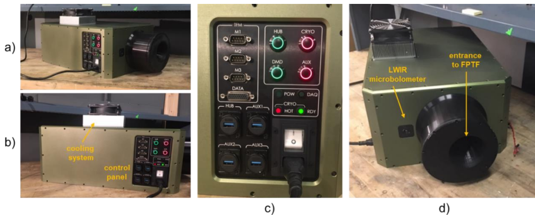
Figure 4. Photographs of the CS-HSI sensor integrated into the environmentally hardened housing, highlighting a) the entire sensor, b) the cooling system and control panel, c) a close-up of the external control panel, and d) the entrance to the FPTF and the LWIR context camera.
