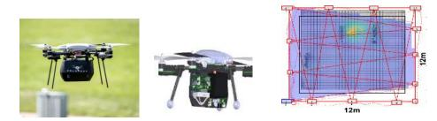
Fig. 3 – Small (24") UAV with b-TDLAS payload aimed at ground; Raster-scan flight pattern and plume image
