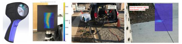
Figure 1: (left) Concept rendering of the RMLD-QGI, (center, left) image of methane plume from a Hencken burner, (center, right) breadboard RMLD-QGI transceiver and electronics support van, and (right) first-ever image of fugitive emission from a residential gas leak.
