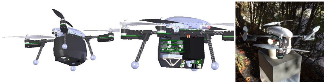
Figure 2. Backscatter Laser Sensor and Small UAV system the RMLD-UAV.
