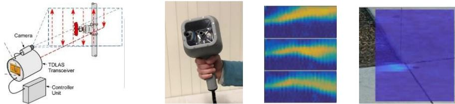
Figure 2 – QGI Concept; Prototype Handheld Transceiver; Successive 1-second images of a 15 scfh methane plume at 3 m distance; Small leak emanating from a sidewalk.
