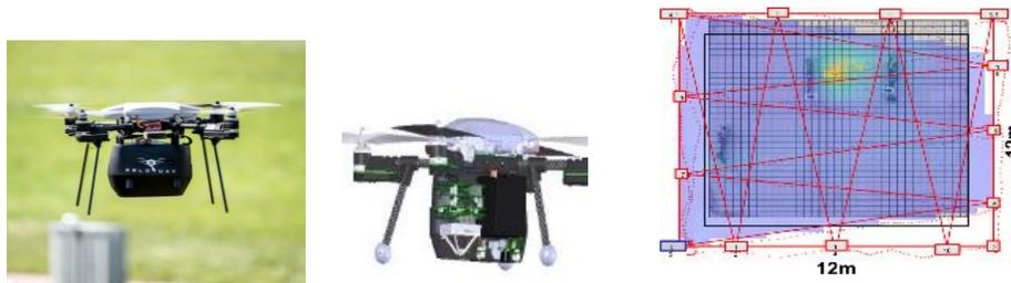
Fig. 3 – Small (24”) UAV with b-TDLAS payload aimed at ground; Raster-scan flight pattern and plume image
