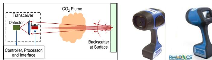
Fig. 1 - Backscatter TDLAS, underlying the Remote Methane Leak Detector (RMLD®), measures methane column density.
