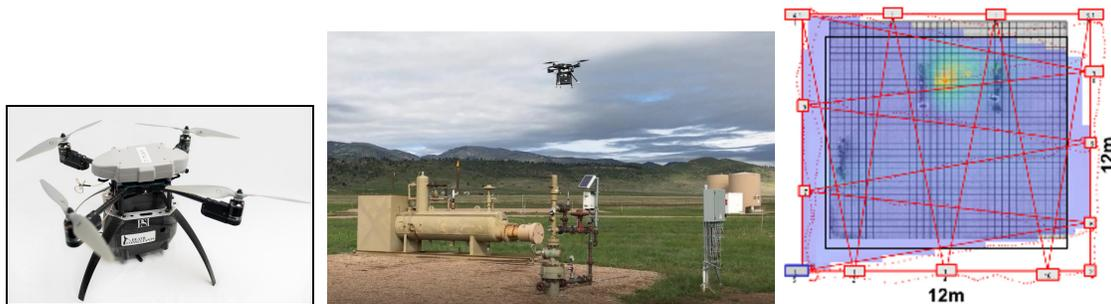
Figure 1: (left) RMLD-UAV, (center) flight at simulated experimental gas wellpad, and (right) flight pattern for surveying a wellpad and data visualization produced.
