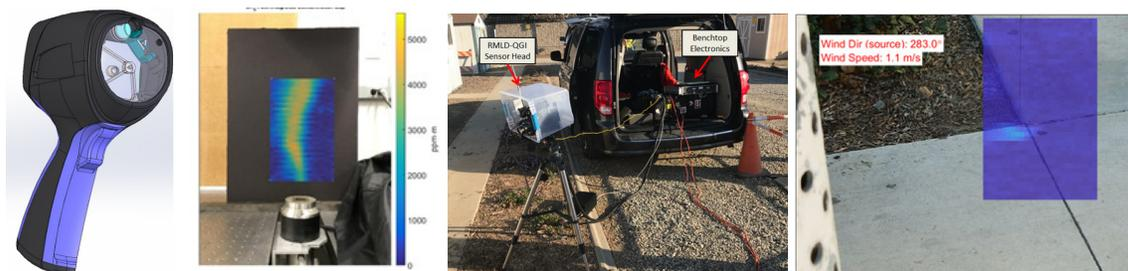
Figure 1: (left) Concept rendering of the RMLD-QGI, (center, left) image of methane plume from a Hencken burner, (center, right) breadboard RMLD-QGI transceiver and electronics support van, and (right) first-ever image of fugitive emission from a residential gas leak.
