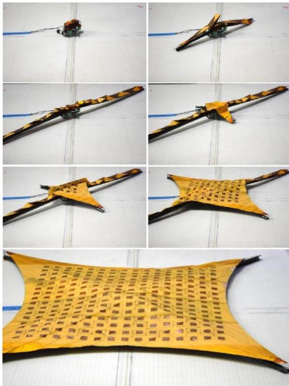
**Figure 5: Sequential deployment of 16x16 element antenna**
