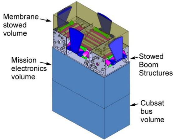
**Figure 2: Layout of system in stowed configuration**
