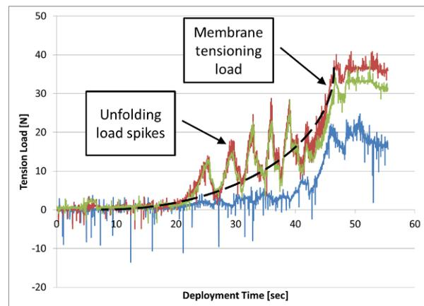
**Figure 4: Deployment drag over the course of the simultaneous deployment of the 16x16 element antenna**
