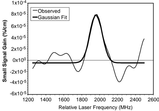
**Figure 14. Processed tunable diode laser scan of atomic iodine line, showing net positive gain: 5% O<sub>2</sub>/Ar, 70 W, 1.5 torr, 7 ms reaction time, NO<sub>2</sub> added, [O] ≅ [I<sub>2</sub>]<sub>0</sub> = 6 x 10<sup>12</sup> cm<sup>-3</sup>, O<sub>2</sub>(a) yield = 0.25. A Gaussian fit to the data is also shown.**
