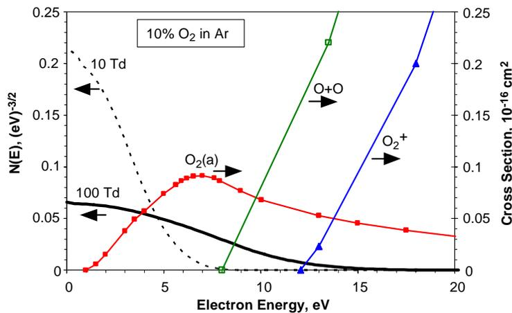
**Figure 2. Illustration of overlap of electron energy distributions with electron impact excitation cross sections for O<sub>2</sub>(a) excitation, O<sub>2</sub> dissociation to form O + O, and O<sub>2</sub> ionization to form O<sub>2</sub><sup>+</sup>. The electron energy distributions are computed for E/N = 10 and 100 Td, in 10% O<sub>2</sub>/Ar. Cross section values were taken from Ref. 20.**
