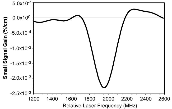
**Figure 12. Processed tunable diode laser scan from the data in Figure 11, 5%  $O_2/Ar$ , 70 W, 1.5 torr, 13 ms reaction time.**
