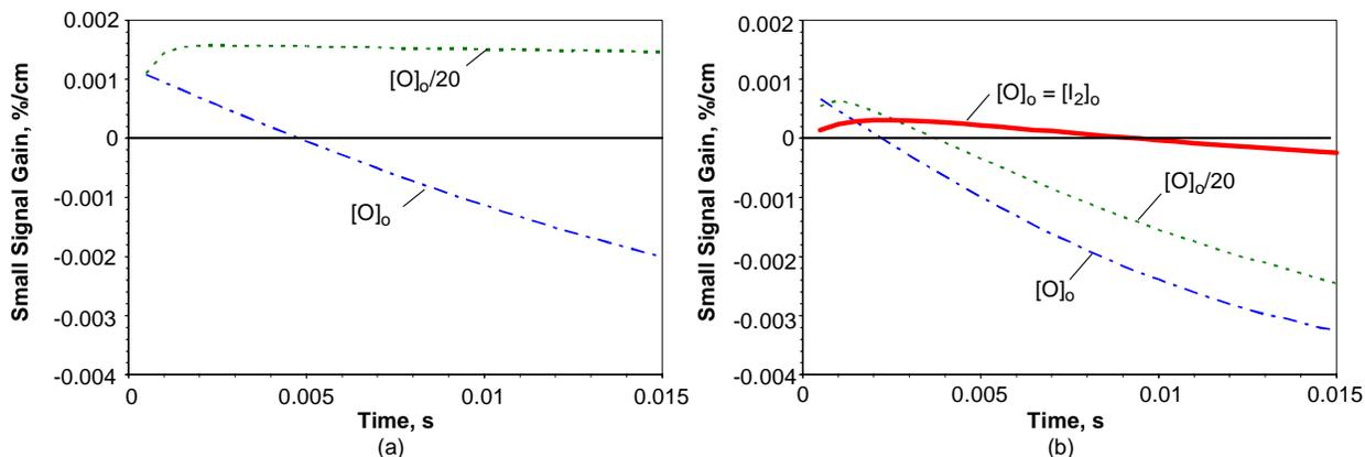
**Figure 17.** Dependence of small-signal gain on reaction time, computed for the reaction mechanism given in Table 1, 5% O<sub>2</sub>/Ar, 1.5 torr, 350 K, initial O<sub>2</sub>(a) yield = 0.23, initial O yield = 0.3: (a)  $k_4 = k_{-4} = k_5 = 0$ ,  $k_6 = 1 \times 10^{-11} \text{ cm}^3/\text{s}$ ; (b) rate coefficients as given in Table 1 with  $k_4 = 7 \times 10^{-12} \text{ cm}^3/\text{s}$ .
