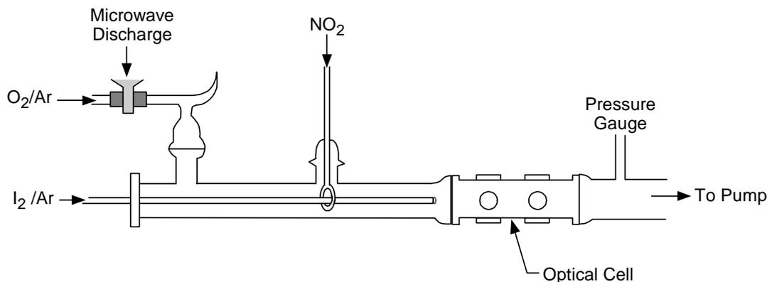
**Figure 4. Schematic diagram of discharge-flow reactor apparatus.**
