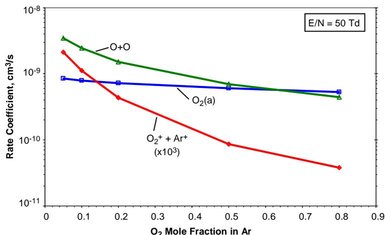
**Figure 3. Effect of variations in O<sub>2</sub> mole fraction on computed electron-impact rate coefficients for O<sub>2</sub>(a) excitation, O<sub>2</sub> dissociation, and total ionization for discharge-excited O<sub>2</sub>/Ar mixtures, E/N = 50 Td.**
