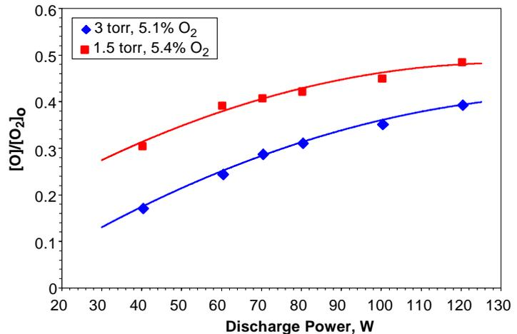
Figure 6. Dependence of atomic oxygen yield on microwave discharge power for 1.5 and 3 torr, ~5%  $O_2$  in Ar.
