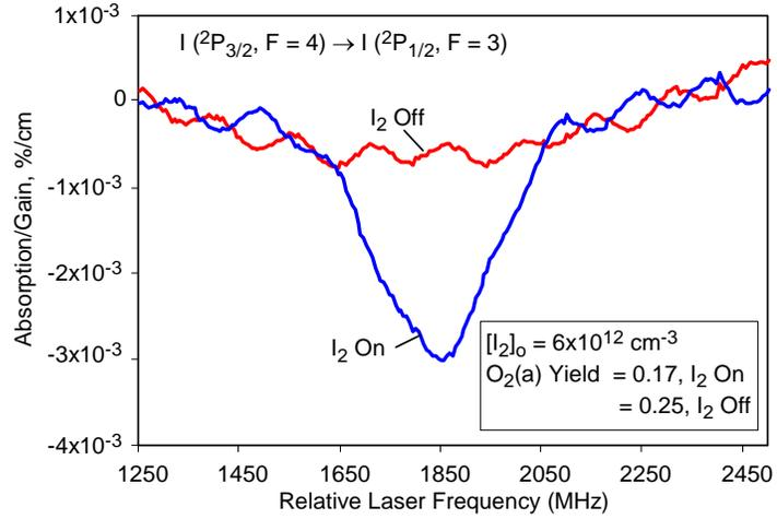
**Figure 11. Single-pass tunable diode laser scans of atomic iodine line in net absorption, with and without the addition of  $I_2$ : 5%  $O_2/Ar$ , 70 W, 1.5 torr, 13 ms reaction time.**
