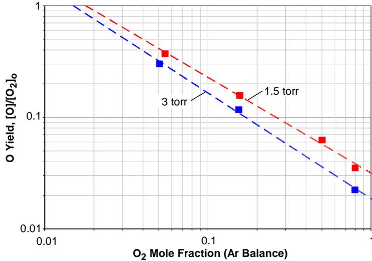
**Figure 7. Dependence of atomic oxygen yield on O<sub>2</sub> mole fraction and total pressure: Ar diluent, 70 W discharge power, 1.5 and 3 torr.**
