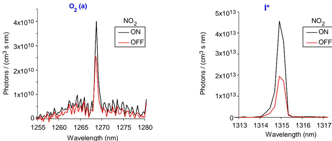
**Figure 13.** Effect of  $NO_2$  addition on observed  $O_2(a) \rightarrow X$  and  $I^* \rightarrow I$  emission intensities: 5%  $O_2/Ar$ , 110 W, 1.5 torr,  $[NO_2]_{\text{added}} = 0.95[O]_o$ ,  $[O]/[O]_o = 1/20$ . With  $NO_2$  off:  $O_2(a)$  yield = 0.15,  $[I^*]/[I] = 0.13$ . With  $NO_2$  on:  $O_2(a)$  yield = 0.25,  $[I^*]/[I] = 0.36$ .
