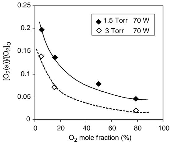
**Figure 8. Dependence of O<sub>2</sub>(a) yield on O<sub>2</sub> mole fraction and total pressure: Ar diluent, 70 W discharge power, 1.5 and 3 torr.**
