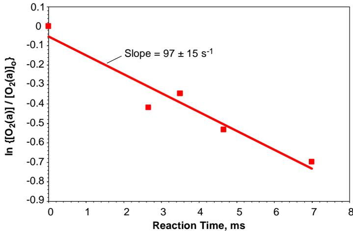
**Figure 15. O<sub>2</sub>(a) decay and first-order loss rate upon addition of I<sub>2</sub>: [I<sub>2</sub>]<sub>0</sub> = 4.7 x 10<sup>12</sup> cm<sup>-3</sup>, 5.5% O<sub>2</sub>/Ar, 70 W, 1.58 torr, [O<sub>2</sub>(a)]<sub>0</sub> = 6 x 10<sup>14</sup> cm<sup>-3</sup>.**
