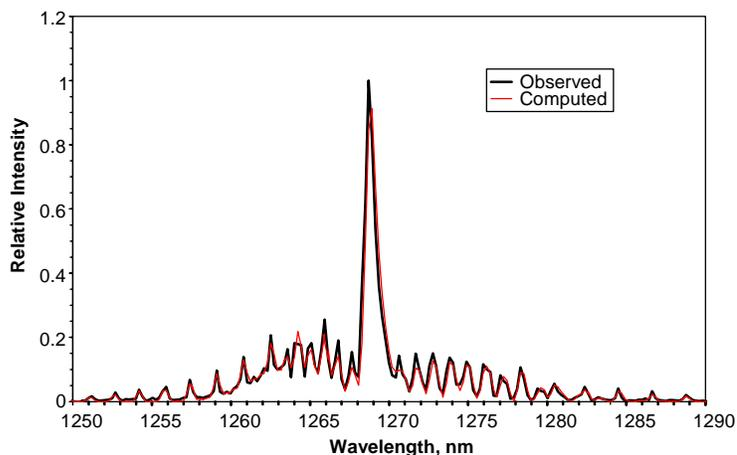
**Figure 5. Observed and best-fit computed spectra for  $\text{O}_2(a \rightarrow X)$  emission: microwave discharge of  $\text{O}_2$  at 2.6 torr, spectral resolution 0.5 nm, rotational temperature 350 K.**
