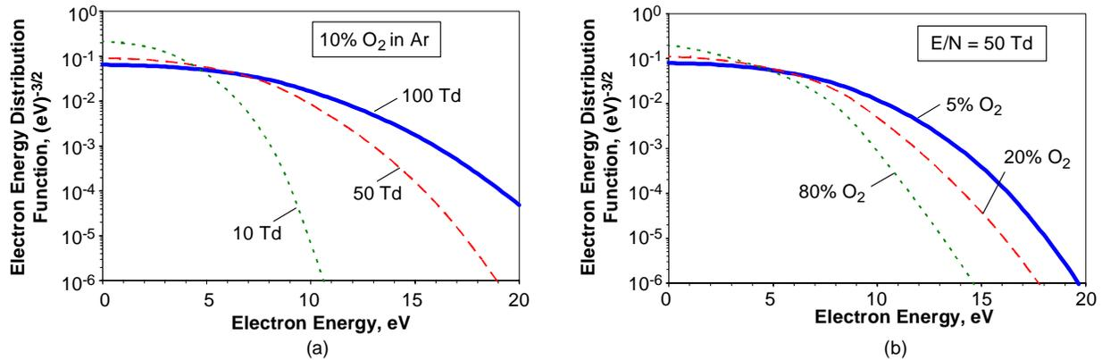
**Figure 1. Computed electron energy distribution functions in discharge-excited O<sub>2</sub>/Ar mixtures: (a) Effect of variations in E/N for 10% O<sub>2</sub> in Ar; (b) Effect of variations in O<sub>2</sub> mole fraction for E/N = 50 Td.**
