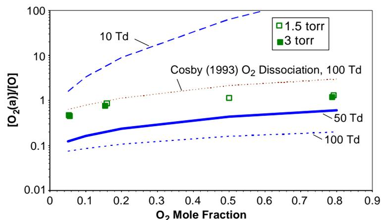
**Figure 10.** [O<sub>2</sub>(a)]/[O] ratios observed at 1.5 and 3 torr, compared to computed upper bounds as described in the text.
