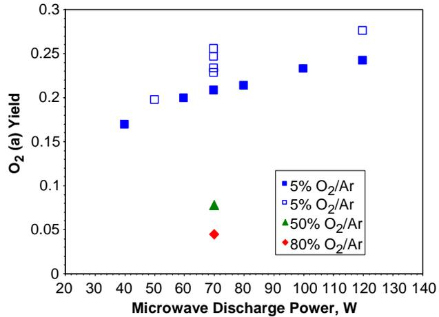
**Figure 9. Dependence of O<sub>2</sub>(a) yield on microwave discharge power for 1.5 torr and three O<sub>2</sub>/Ar mixtures. The two data sets for 5% O<sub>2</sub>/Ar were observed on separate, consecutive days, and indicate day to day variability in the discharge operation.**
