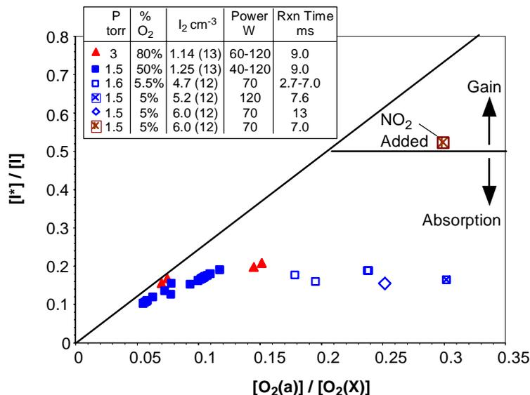
**Figure 16.** Observed dependence of  $[I^*]/[I]$  on  $[O_2(a)]/[O_2(X)]$ , compared to the equilibrium relationship. Inversion of the atomic iodine state populations and positive gain occur for  $[I^*]/[I] > 0.5$ .
