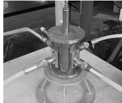
**Figure 7. The solar receiver housing with four fiber cables connected.**
