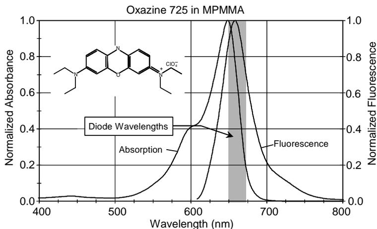
Figure 1: Normalized absorption and emission spectra of Ox 725 in MPMMA.
