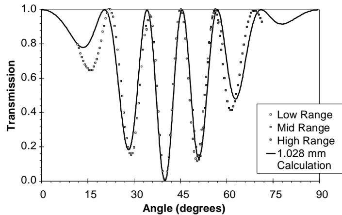
Figure 5: Comparison of experimental results and calculation for the transmission of polarized 633-nm light through the crystal quartz BRF. The agreement is excellent over the central ( $30^\circ$  to  $60^\circ$ ) region of the curve that is useful for tuning.
