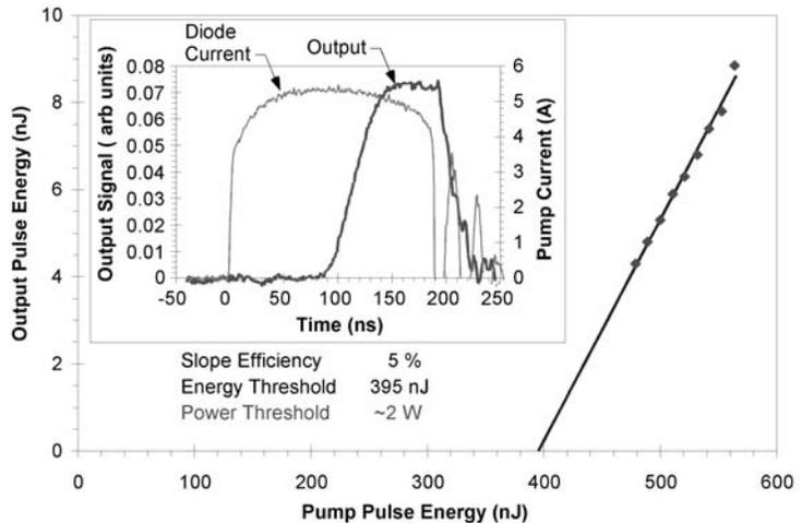
Figure 17: Unoptimized input/output curve for the brassboard diode-pumped tunable SSDL ( $R_{OC} = 98\%$ ). Typical temporal profiles for the diode current pulse and SSDL output are shown in the inset. The gain medium is Ox 725 (3 mM) in MPMMA.
