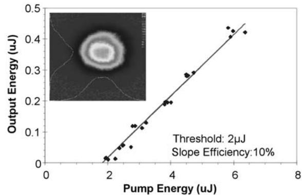
Figure 14: I/O curve for the brassboard solid-state dye laser with  $R_{OC} = 98\%$  and the output tuned to 725 nm.
