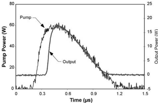
Figure 10: Very good temporal tracking is observed between the pump and output pulse over a tuning range from  $\approx 710$  to  $\approx 750$  nm. A single output wavelength is observed in this spectral region.
