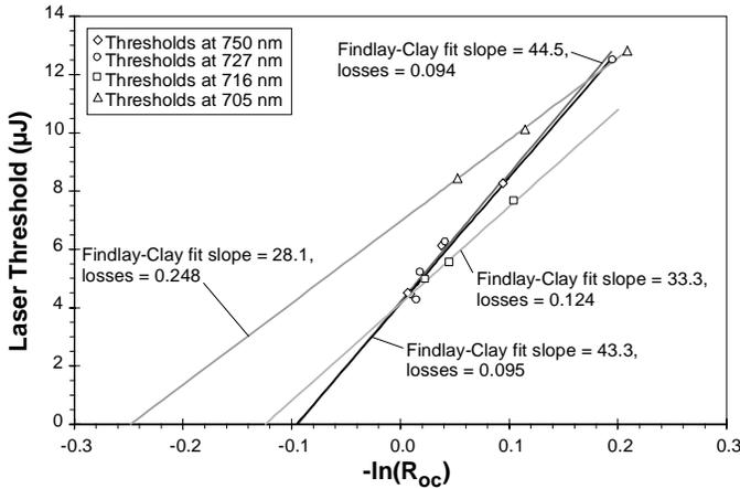
Figure 9: Findlay-Clay analyses for sample PSIN-017 in the three-mirror resonator at four wavelengths: 705, 716, 727 and 750 nm. The round-trip cavity loss increases as the output wavelength is tuned towards the peak absorption of the dye ( $\approx 650$  nm).
