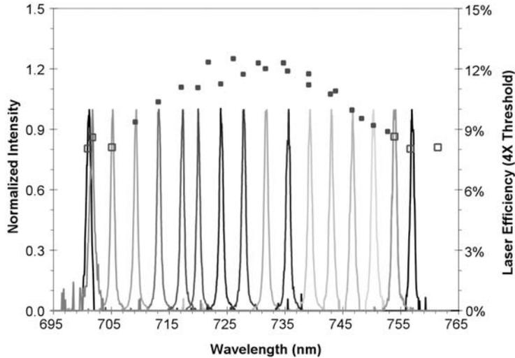
Figure 13: Normalized spectral data collected using a BRF in the three-mirror resonator of Figure 2. The peaks are separated by  $\approx 3.7$  nm, and each peak has a FWHM of  $\approx 0.8$  nm. The squares are laser efficiency data taken at 4x threshold and plotted on the right-hand axis. The efficiencies recorded at points where two output wavelengths were observed are displayed as open squares.
