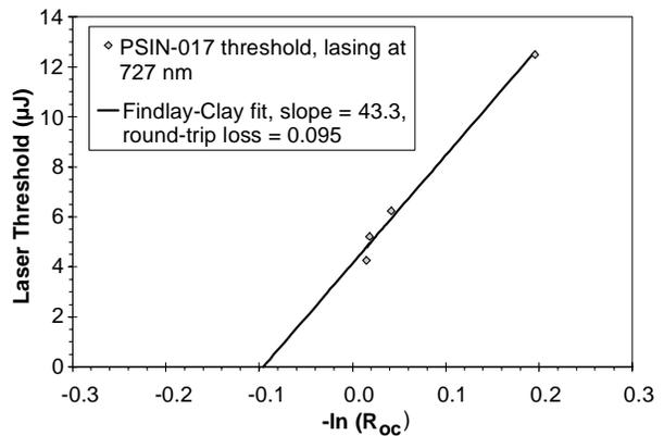
Figure 8: Findlay-Clay analysis for sample PSIN-017 tuned to 727 nm in three-mirror resonator.
