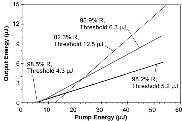
Figure 7: Energy I/O curves for the tuned resonator ( $\lambda \approx 727$  nm) for several output couplers. The legend identifies the output-coupler reflectivity for each data set and also reports the laser threshold. The actual data points are omitted for clarity. The sample is PSIN-017.
