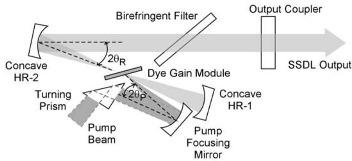
Figure 2: Resonator design for the tunable solid-state dye laser. The tuning element is the birefringent filter in the collimated section.
