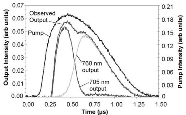
Figure 11: Temporal traces showing the pump profile (left axis) and the output profiles (right axis) for tuning at the extremes of the wavelength range. The observed output was resolved into two components at different wavelengths.
