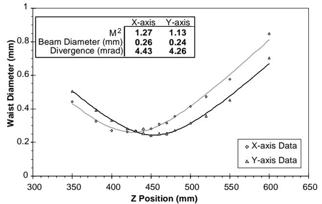
Figure 16: Beam quality measurements for the brassboard SSDL operated at  $\approx 3 - 4\times$  threshold. The values yielding the best fit for each data set are shown in the inset.
