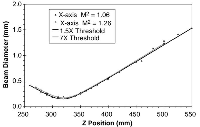
Figure 12: Beam quality measurements for the three-mirror SSDL. From these data, the  $M^2$  value is  $\cong 1.06$  near threshold. When well above threshold, the  $M^2$  value degrades slightly to  $\cong 1.26$ .
