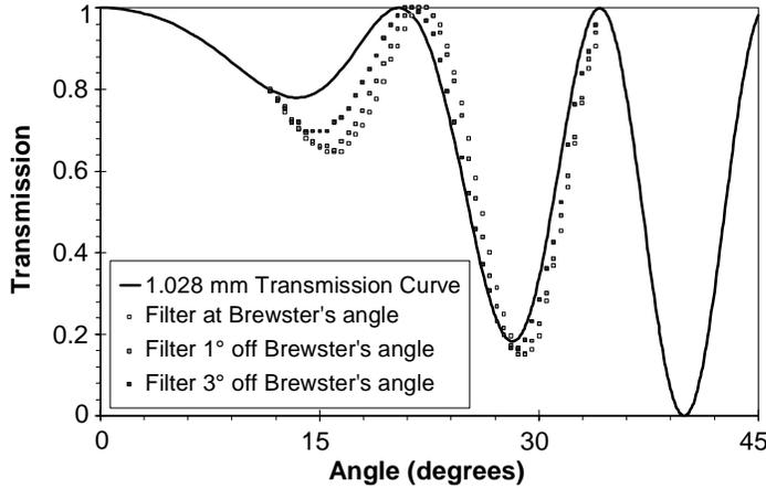
Figure 6: Effect on the BRF transmission curve as the angle of incidence is adjusted away from Brewster's angle. The effect is small except for angles below 20°. The best angles for laser tuning are in the range of 30° to 60°, because of the high rejection ratios.
