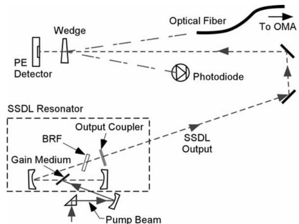
Figure 3: The optical layout of the diagnostics for the SSDL output.
