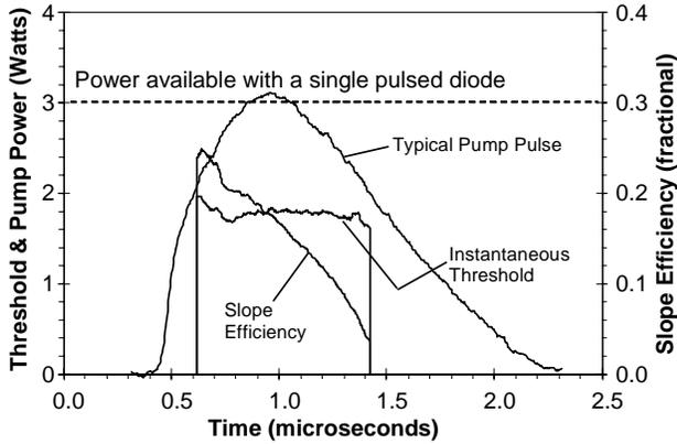
Figure 15: Time-resolved I/O data for the brassboard solid-state dye laser with  $R_{OC} = 98\%$  and the output tuned to 725 nm. The threshold power is constant at  $\approx 2\text{W}$  during the pulse. This is below the peak power available from the pulsed diode laser.
