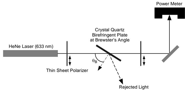
Figure 4: Experimental layout for measuring the transmission of the BRF tuner. (The black arrows indicate the polarization direction that is passed.) The BRF is rotated about its axis of symmetry, and the transmitted light is recorded as a function of this angle.
